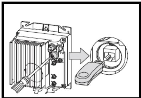
Figure 3: Bluetooth connection to RASP5
