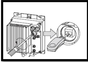
The drivesConnect mobile App helps to connect smartphone to the RASP5. The parametrization and monitor information can be done by using the App (Android or IOS based). For detailed information refer to Appnote: APO40189EN in the [Overview Drives Appnotes](#)
