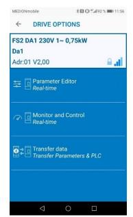
On the device itself you can read or write parameter, control or monitor in real-time and transfer parameter sets or PLC data.
