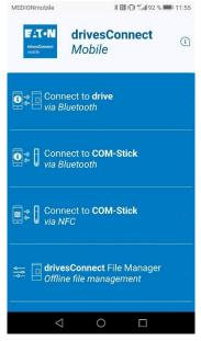
Choose "Connect to drive via Bluetooth". Therefor the drive needs to be insert in a powered PowerXL device.
