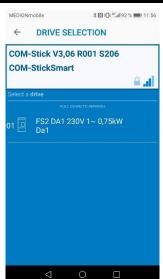
After it you can choose the PowerXL device you want to parameterize or control. If a couple of devices are linked together, you can reach all devices with one DX-COM-STICK3.
