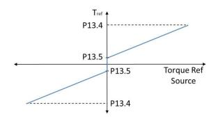
When, for example, an analog signal 0 ... 10 V is used as torque reference, 0 V corresponds to the value set with P13.5 and +10 V to the one set with P13.4.
