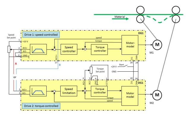
Motor M1 determines the line speed. The speed set point comes from a potentiometer and is connected to analog input Al1. Motor M2 is torque controlled and defines the tension of the material. In case the torque (tension) is set too high, it is possible than motor 2 tries to accelerate motor 1, which must be able to brake in this situation.
