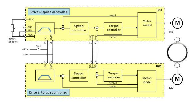
Motor M1 is speed controlled. The speed set point is defined by a potentiometer, which is connected to analog input Al1. The torque reference of drive 1 is also used as torque reference for drive 2, using analog output AO1 of drive 1 and analog input Al2 of drive 2. Ramp and speed controller of drive 2 are not used. Because the two motors are coupled mechanically, no speed supervision for drive 2 is necessary.
