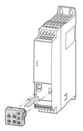
DXE-EXT-SET is an optional module, which can be plugged onto the front of the Variable Speed Starter. It is used for simple modification of selected parameters without using a PC or keypad. All sizes of DE1 use the same module.
