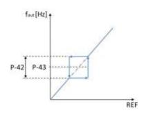
Fading out frequencies is possible with all kind of reference signals, not depending on where they come from, e.g. analog input, fixed frequency, digital reference ... , whatever is selected.
