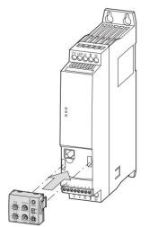
DXE-EXT-SET is an optional module, which can be plugged onto the front of the Variable Speed Starter. It is used for simple modification of selected parameters without using a PC or keypad. All sizes of DE11 use the same module.
