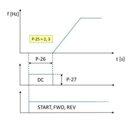
Parameter P-25 "DCBrake" determines, in which situations a DC braking is performed. In case the braking is required before starting, P-25 has to be set to 2 or 3.
