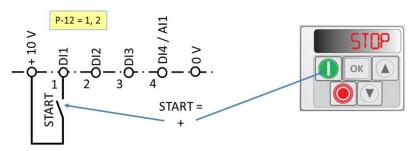
The drive starts with the ramp defined by P-03 "t-acc". Pushing the STOP button or removing the signal at terminal 1 leads to a stopping. The behavior depends on the setting of P-05 "Stop Mode".
