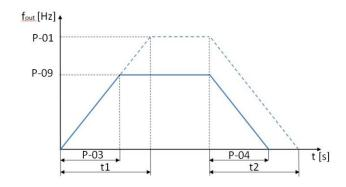
In most cases the rated frequency of the motor (P-09) is equal to the max frequency (P-01). In case a motor is operated above its rated speed, this has to be taken into account when setting the ramp times.
