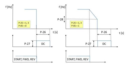
Parameter P-25 "DCBrake" determines, in which situations a DC braking is performed. In case a DC braking is required at stop, P-25 has to be set to 1 or 3.
