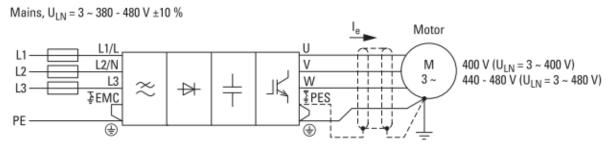
When applying the supply voltage, the d.c. link capacitor will be charged. Current limiting elements are used to prevent an inrush peak of the current. After the charging, the elements are bypassed. They are not effective during operation. It has to be noted that the current limiting elements are not foreseen for a continuous duty. Therefore the number of starts per time is limited. Typical value: 1 charging per 30 s.
