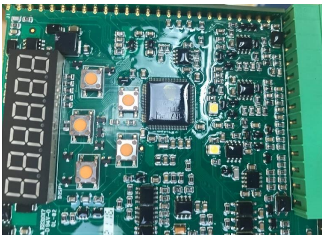
Example of an Eaton PCB with machine applied conformal coating.
