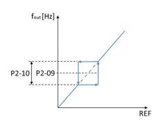
Fading out frequencies is possible with all kind of reference signals, not depending on where they come from, e.g. analog input, fixed frequency, output of a PI controller, digital reference ..., whatever is selected.
