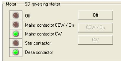
Figure 32: Status display of the motor starter contactors
