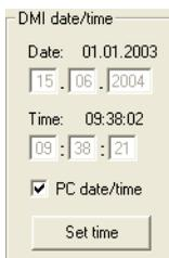
Figure 34: Display of the currently set date and time in the DMI
