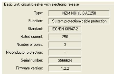
Figure 14: Device data of a circuit-breaker with electronic release
