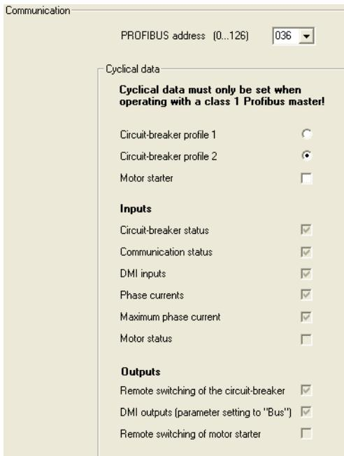
Figure 10: Setting the PROFIBUS address of the DTM
