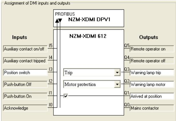
Figure 30: Example of an assignment of the free inputs/outputs
