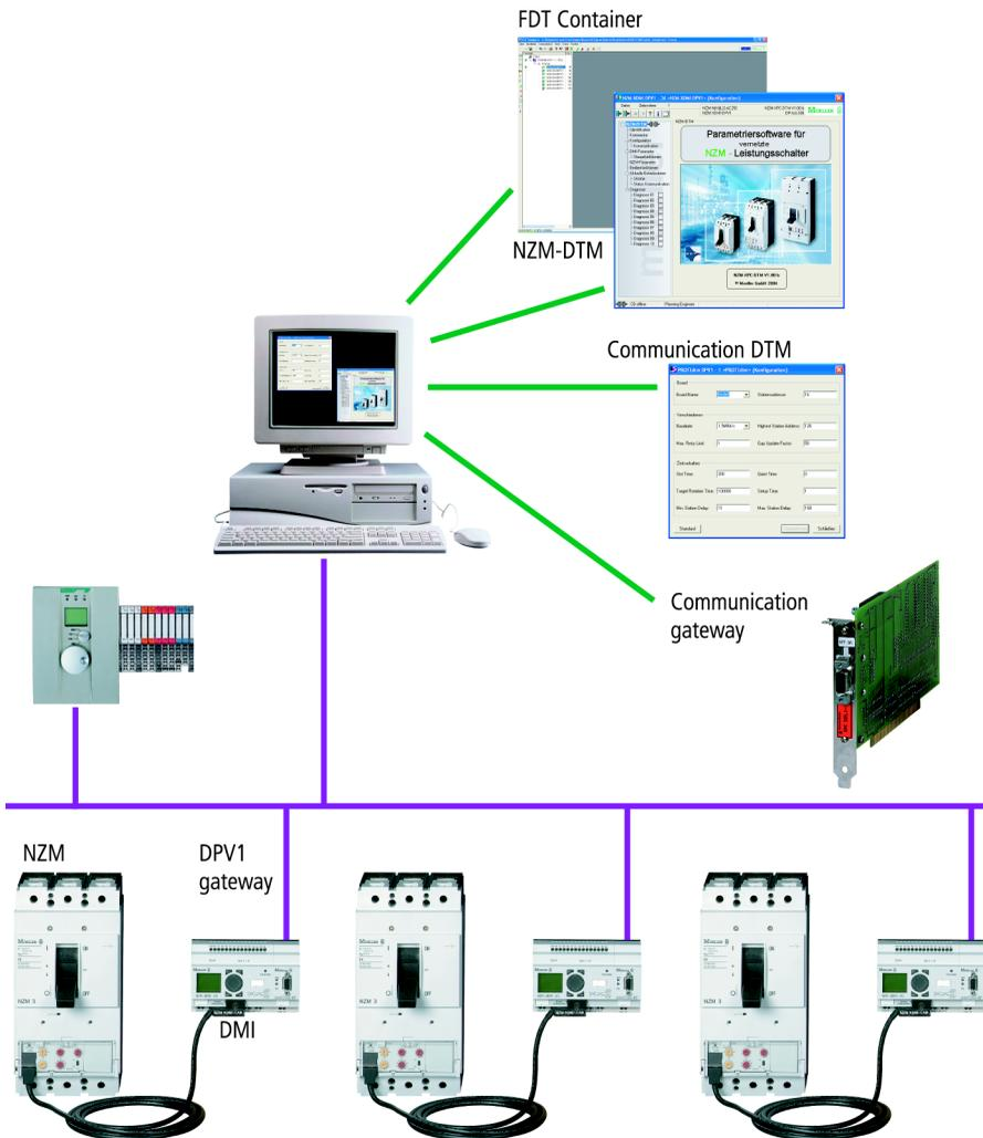
Figure 1: Example of a system for the parameter setting and diagnostics of NZM circuit-breakers
