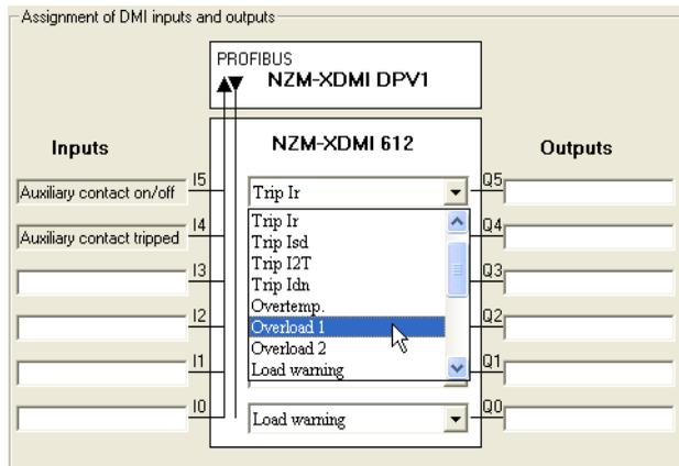
Figure 29: Condition for setting a DMI output
