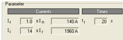
Figure 45: Working parameters of the circuit-breaker electronics at the time of a status change
