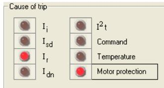
Figure 43: Cause of circuit-breaker trip
