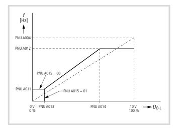
Figure 50: Setpoint matching, terminals O–L
