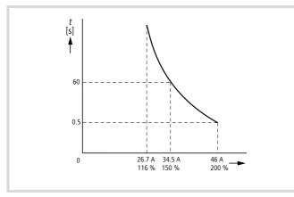
Figure 120: Example of tripping characteristic using a DV6-340-11K with the tripping current set at 46 A
