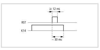
Figure 69: Function chart for RST (reset) K14: Signalling relay contact K14
