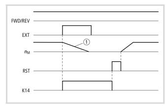
Figure 65: Function chart for EXT (external fault message)
