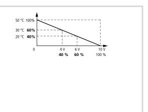
Figure 144: Example of temperature control
