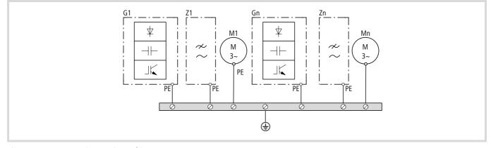
Figure 14: Star-type point-to-point earthing
