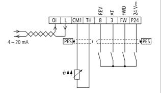
Figure 45: Analog setpoint definition
