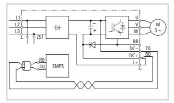
Figure 163: Connecting terminals R0 and T0 to DC+ and DC– SMPS: DV6 control electronics
