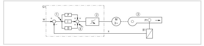
Figure 133: PID control block diagram
