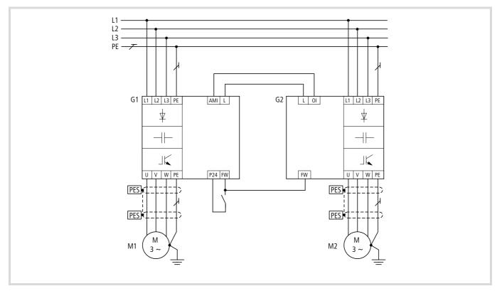
Figure 94: Controlling two motors with two frequency inverters
