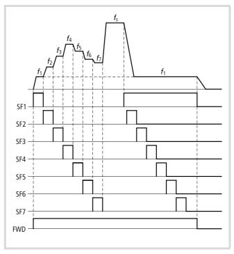
Figure 58: Function chart for SF1 to SF7 (bitwise fixed frequency selection)
