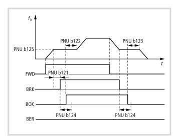
Figure 97: Brake control function chart
