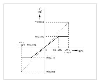
Figure 52: Setpoint matching, terminals O2-L
