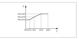
Figure 156: Adjustable overload protection (PNU b013 = 02)
