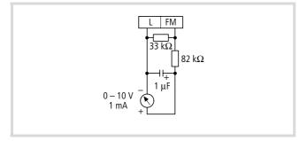
Figure 48: Example for a low-pass circuit
