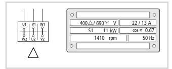
Figure 29: Example in motor delta circuit
