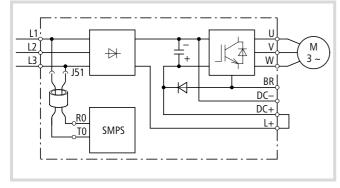
Figure 162: Default connection of terminals R0 and T0 SMPS: DV6 control electronics
