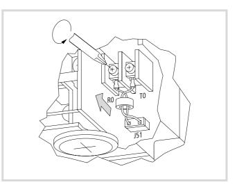
Figure 164: Disconnect J51 from terminals R0 and T0
