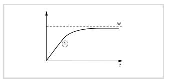
Figure 139: Slow control, large static system deviation
