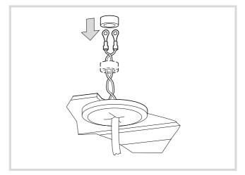
Figure 24: Push on the ferrite rings
