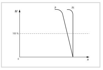
Figure 93: Function chart for PI and P control
