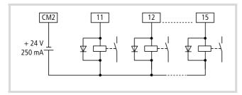
Figure 35: Relay with free-wheel diode
