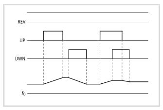
Figure 76: Function chart for UP/DWN (acceleration/deceleration – motor potentiometer)
