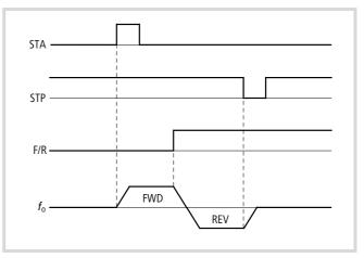
Figure 90: Function chart for STA (pulse start) STP (pulse stop) and F/R (direction reversal)
