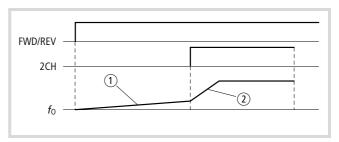
Figure 61: Function chart for 2CH (second acceleration time)
