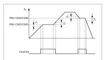
Figure 102: Function chart for FA3 (frequency reached)/FA5
