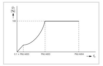
Figure 125: Quadratic  $\Delta UIf$  characteristic  $\Delta U_2$ :Output voltage  $f_0$ : Output frequency
