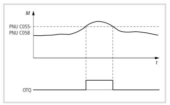
Figure 113: Function chart for OTQ (torque exceeded)
