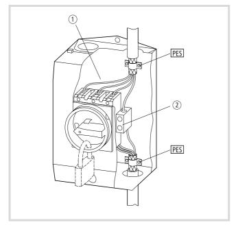
Figure 17: Maintenance switch, e.g. T... in an enclosure
