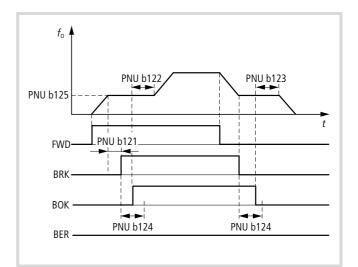
Figure 171: Brake control function chart
