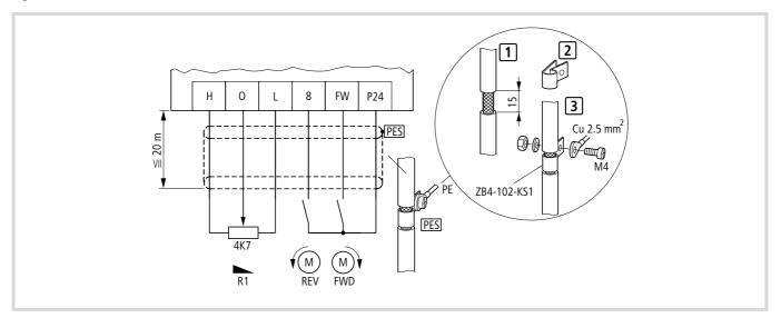
Figure 34: Control terminal connection (factory setting)
