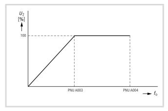
Figure 124: Linear  $\Delta Ulf$  characteristic  $\Delta U_2$ :Output voltage  $f_0$ : Output frequency
