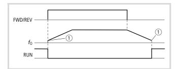
Figure 104: Function chart for RUN (Run signal)
