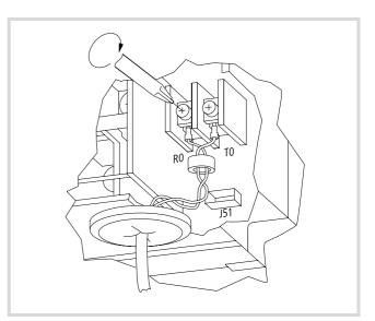
Figure 25: Connecting the external supply voltage
