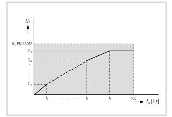
Figure 127: Limits of the freely adjustable  $\Delta UIf$  characteristic
