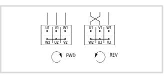
Figure 30: Direction of rotation, change of direction
