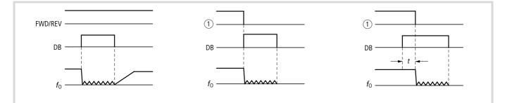
Figure 79: Function chart for DB (DC braking)
