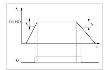
Figure 99: Function chart for FA1 (frequency reached)
