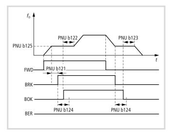
Figure 111: Brake control function chart
