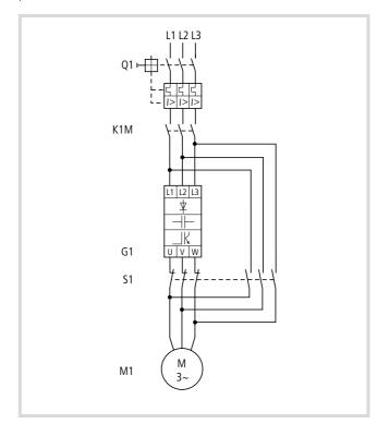
Figure 32: Bypass motor control
