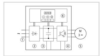
Figure 5: Function chart of the frequency inverter
