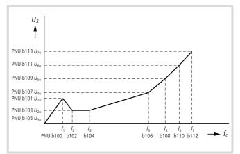
Figure 126: Adjustable *AUIf* characteristic
