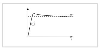
Figure 138: Good control characteristics
