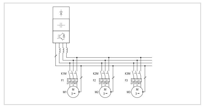
Figure 31: Parallel connection of multiple motors
