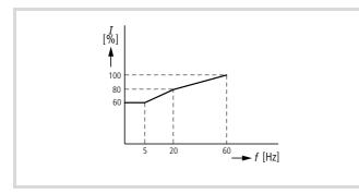
Figure 154: Increased overload protection (PNU b013 = 00)
