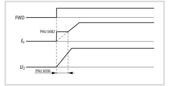
Figure 168: Function chart for starting frequency
