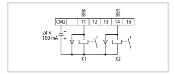
Figure 110: Digital output 11 configured as BRK (release brake) and 14 as BER (brake fault).
