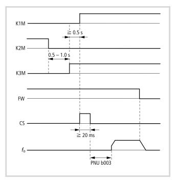
Figure 83: Function chart for CS (heavy mains starting)
