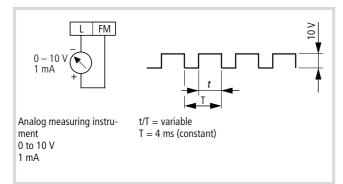
Figure 47: Connection of analog measuring instrument
