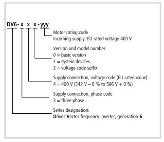
Figure 2: Type codes of the DV6 frequency inverters
