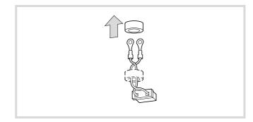
Figure 165: Remove the ferrite rings.
