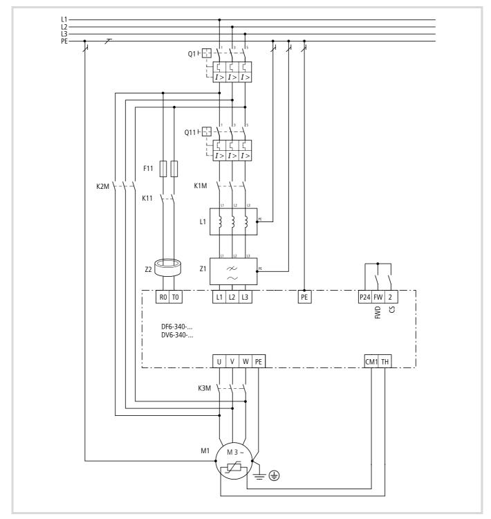
Figure 81: DV6 series frequency inverters with K2M bypass contactor, K3M motor contactor and K1M mains contactor F11: 6 A miniature circuit-breaker, for example FAZ-B6
