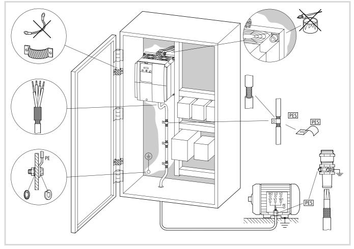
Figure 13: EMC-compliant setup
