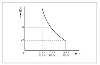
Figure 157: Tripping characteristic for increased overload protection at 20 Hz and  $I_{\rm e}=$  23 A
