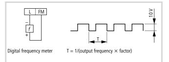
Figure 49: Digital frequency meter connection
