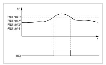
Figure 88: Function chart for torque limits
