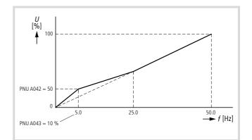
Figure 123: Voltage boost characteristics
