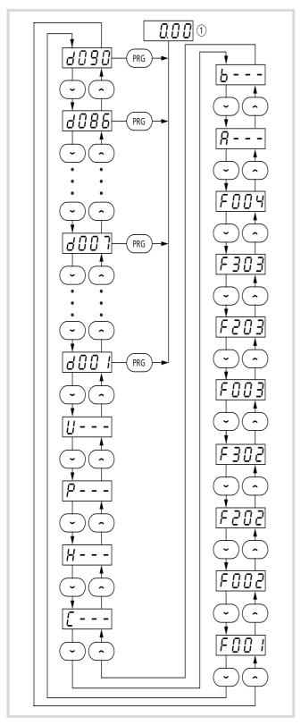
Figure 41: DV6 keypad menu structure
