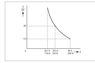
Figure 153: Tripping current characteristic at  $I_e = 23$  A
