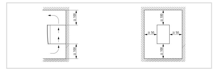
Figure 7: Installation dimensions
