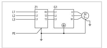
Figure 12: Earthing measures Z1: RFI filter G1: Frequency inverter
