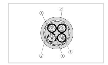
Figure 15: Sample motor cable
