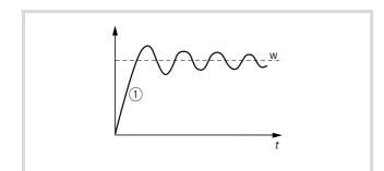
Figure 137: Oscillation, dampened
