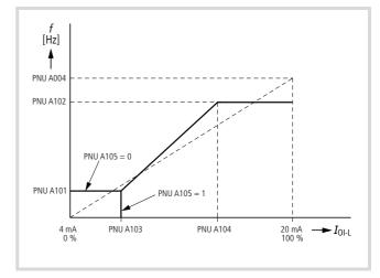
Figure 51: Setpoint current, terminals OI-L
