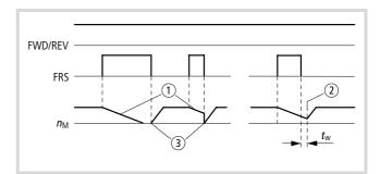
Figure 63: Function chart for FRS (control inhibit and free run stop)  $n_{\rm M}$ : Motor speed
