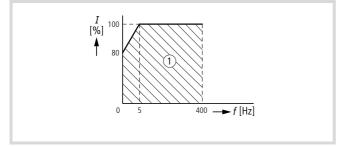
Figure 159: Setting range for the adjustable overload protection (1) Setting range
