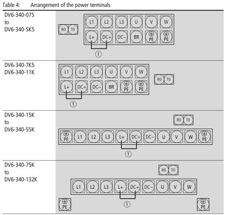
① Internal connection. Remove if a DC link choke is used.
