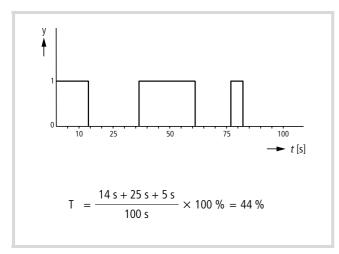
Figure 169: Example: Braking duration
