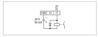
Figure 112: Digital output 11 configured as OTQ (torque exceeded)
