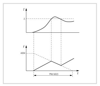
Figure 161: Current limit  $I_{\rm M}$ : Motor current  $I_1$ : Current limit
