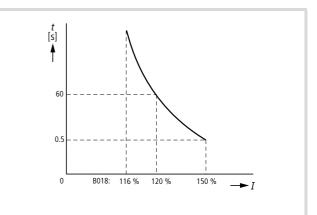
Figure 160: Tripping characteristic for adjustable overload protection using PNU b018
