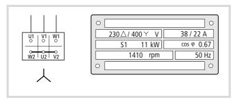
Figure 28: Example in motor star circuit
