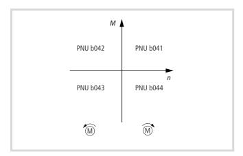
Figure 86: The four quadrants of a motor
