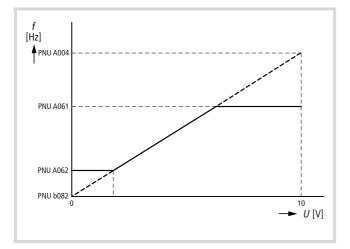
Figure 130: Upper frequency limit (PNU A061) and lower frequency limit (PNU A062)
