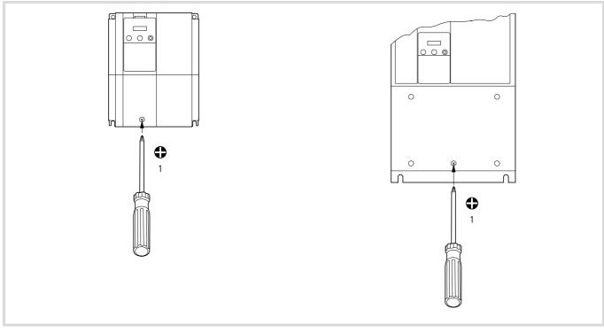
Figure 19: Loosening the screw
