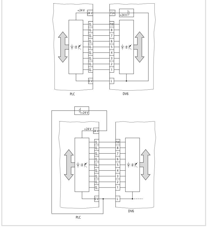
Figure 37: Actuating the digital inputs
