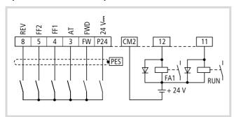
Figure 46: Fixed frequency definition
