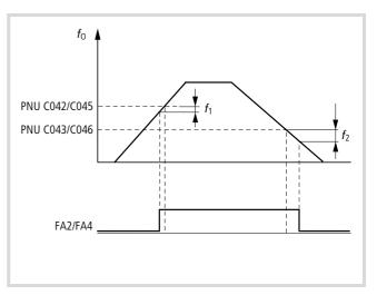
Figure 101: Function chart for FA2 (frequency exceeded)/FA4
