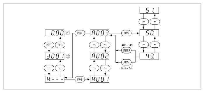
Figure 43: Change the base frequency (example with default setting)
