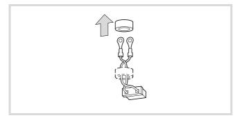
Figure 23: Remove the ferrite rings
