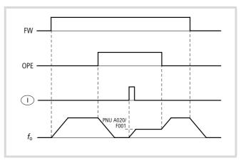
Figure 85: Function chart for OPE (setpoint definition through keypad)
