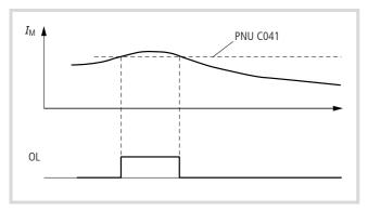
Figure 106: Function chart for OL (overload signal)/OL2
