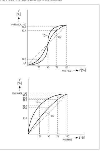
Figure 148: Curvature of the S- and U-curve characteristics
