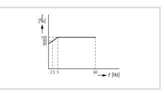
Figure 155: Normal overload protection (PNU b013 = 01)
