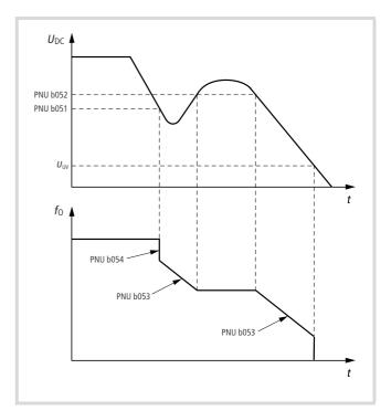
Figure 166: Function chart for controlled deceleration
