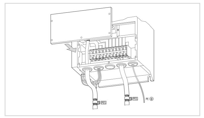
Figure 38: Close the terminal shroud
