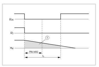
Figure 150: Duration of power supply failure greater than defined under PNU b002
