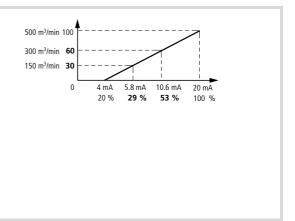
Figure 143: Examples for flow control
