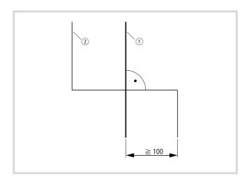
Figure 36: Crossover of signal and power cables
