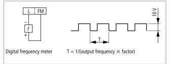
Figure 48: Digital frequency meter connection
