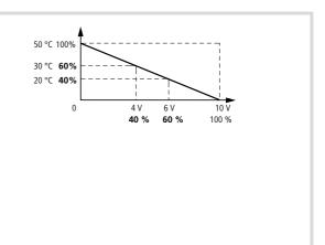
Figure 126: Example of temperature control
