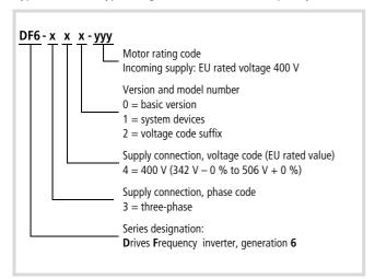
Figure 2: Type codes of the DF6 frequency inverters
