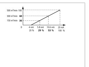
Figure 125: Examples for flow control
