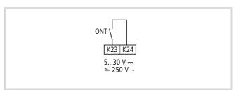
Figure 100: Relay output K23-K24 ONT (Mains On time)
