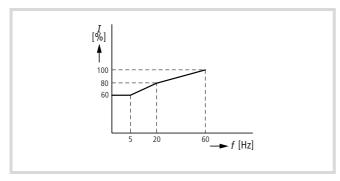
Figure 136: Increased overload protection (PNU b013 = 00)
