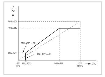
Figure 49: Setpoint matching, terminals O–L
