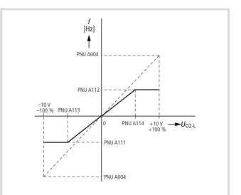
Figure 51: Setpoint matching, terminals O2L
