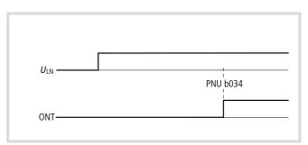
Figure 101: Function chart for ONT (Mains On time)  $U_{LN}$ : Supply voltage
