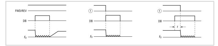
Figure 77: Function chart for DB (DC braking)
