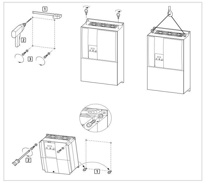
Figure 8: Mounting the DF6
