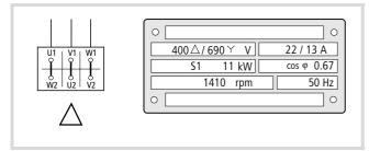
Figure 29: Example in motor delta circuit
