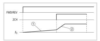
Figure 60: Function chart for 2CH (second acceleration time)
