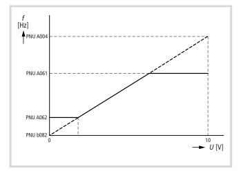
Figure 112: Upper frequency limit (PNU A061) and lower frequency limit (PNU A062)
