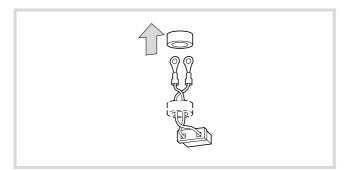
Figure 23: Remove the ferrite rings
