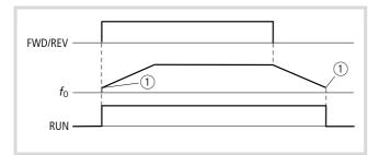
Figure 92: Function chart for RUN (Run signal)
