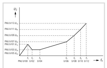
Figure 108: Adjustable UIf characteristic
