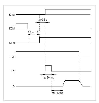
Figure 81: Function chart for CS (heavy mains starting)
