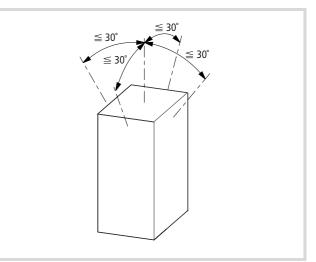
Figure 6: Mounting position
