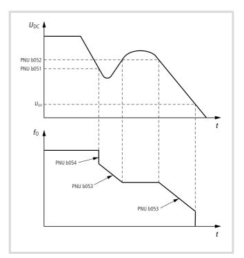
Figure 148: Function chart for controlled deceleration
