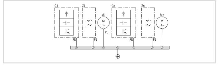
Figure 14: Star-type point-to-point earthing
