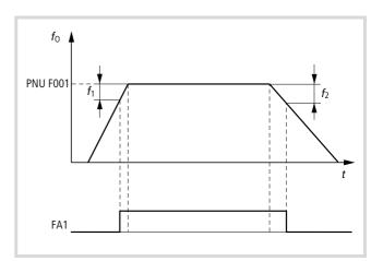
Figure 87: Function chart for FA1 (frequency reached)
