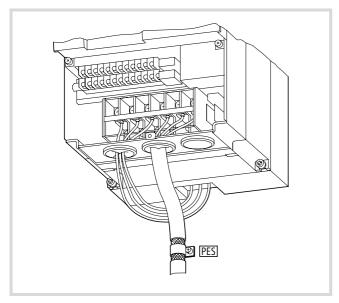
Figure 21: Cable connection to the power terminals
