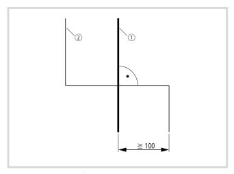
Figure 35: Crossover of signal and power cables
