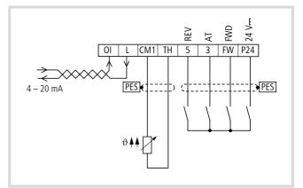
Figure 44: Analog setpoint definition
