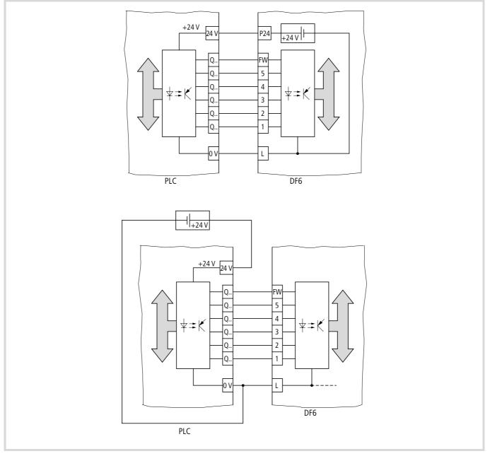
Figure 36: Triggering the digital inputs
