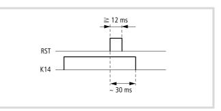
Figure 68: Function chart for RST (reset) K14: Signalling relay contact K14
