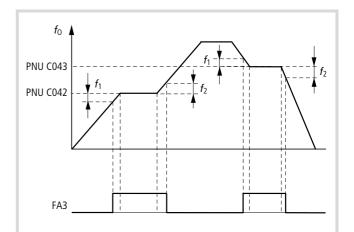
Figure 90: Function chart for FA3 (frequency reached)
