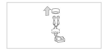
Figure 147: Remove the ferrite rings.
