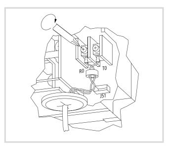
Figure 25: Connecting the external supply voltage
