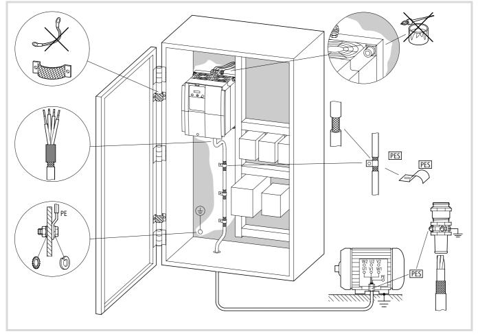
Figure 13: EMC-compliant setup
