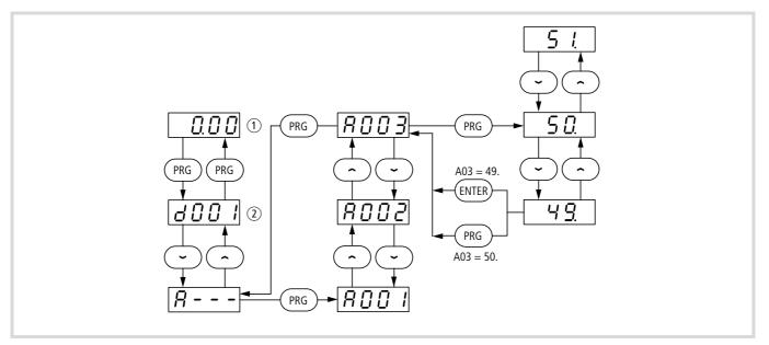
Figure 42: Changing the base frequency (example with default setting)
