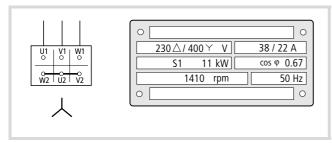
Figure 28: Example in motor star circuit
