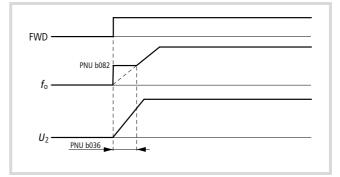
Figure 150: Function chart for starting frequency
