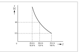
Figure 139: Tripping characteristic for increased overload protection at 20 Hz and  $I_{\rm e}=$  22 A
