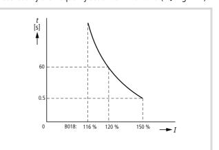
Figure 142: Tripping characteristic for adjustable overload protection using PNU b018
