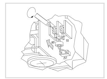
Figure 22: Remove the connection of J51 to R0 and T0
