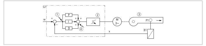
Figure 115: PID control block diagram
