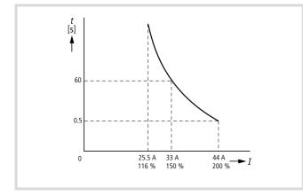
Figure 135: Tripping current characteristic at  $I_e = 22 \text{ A}$
