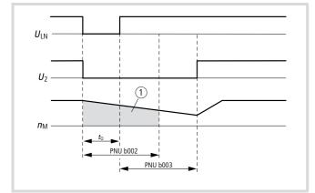
Figure 131: Duration of power failure less than set under PNU b002
