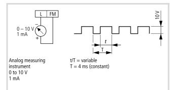
Figure 46: Connection of analog measuring instrument
