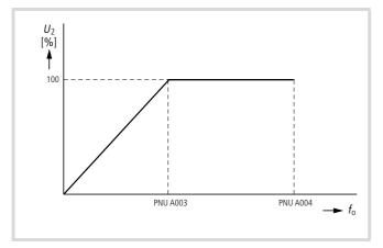
Figure 106: Linear Ulf characteristic
