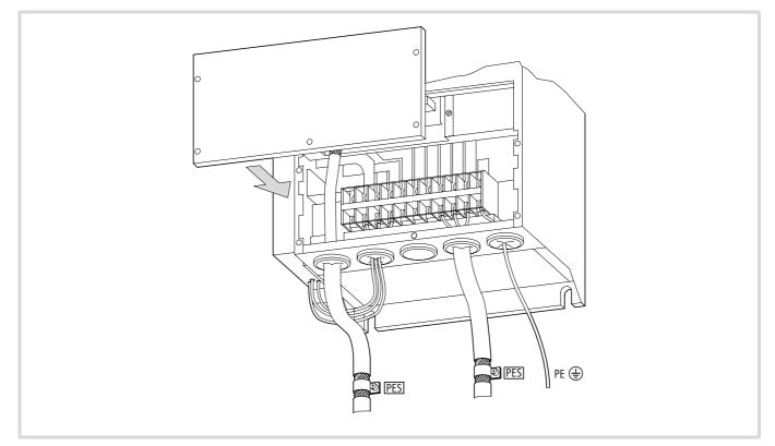
Figure 37: Close the terminal shroud
