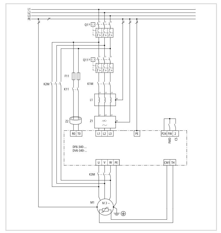
Figure 79: DF6 series frequency inverters with K2M bypass contactor, K3M motor contactor and K1M mains contactor F11: 6 A miniature circuit-breaker, for example FAZ-B6
