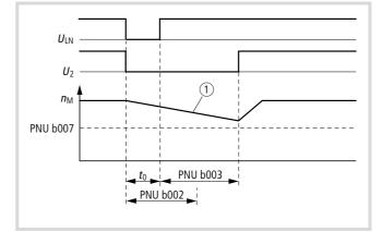
Figure 133: Motor frequency higher than set under PNU b007
