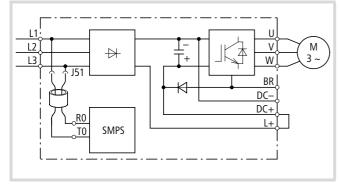
Figure 144: Default connection of terminals R0 and T0 SMPS: DF6 control electronics
