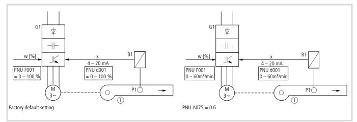
Figure 124: Example for scaling adjustment
