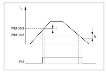
Figure 89: Function chart for FA2 (frequency exceeded) fo:Output frequency
