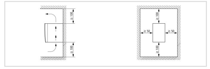
Figure 7: Installation dimensions
