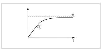
Figure 121: Slow control, large static system deviation w: Setpoint
