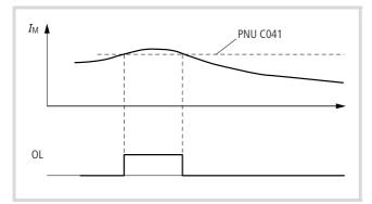
Figure 94: Function chart for OL (overload signal)
