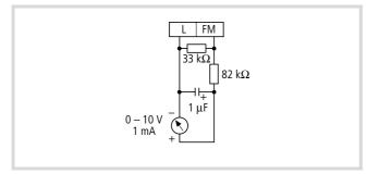
Figure 47: Example of a low-pass circuit
