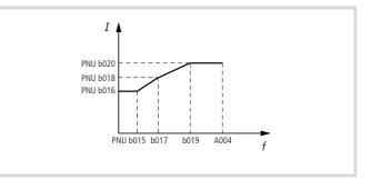
Figure 138: Adjustable overload protection (PNU b013 = 02)
