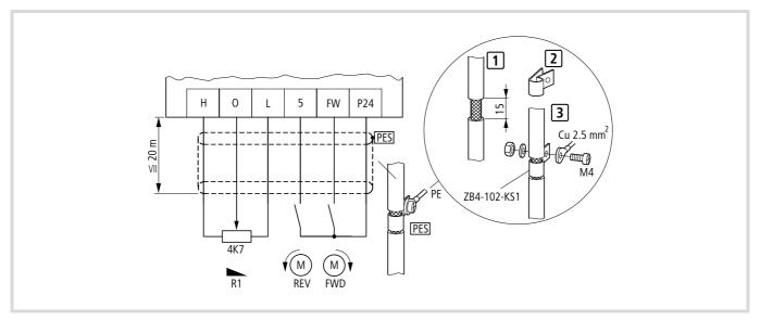
Figure 34: Control terminal connection (factory setting)
