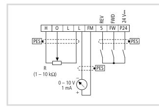
Figure 43: Connecting an external potentiometer
