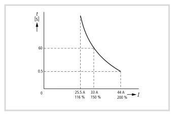
Figure 102: Tripping characteristic using a DF6-340-11K as an example, with the tripping current set to 22 A
