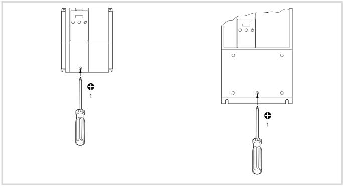
Figure 19: Loosening the screw
