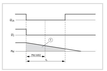
Figure 132: Duration of power failure longer than set under PNU b002
