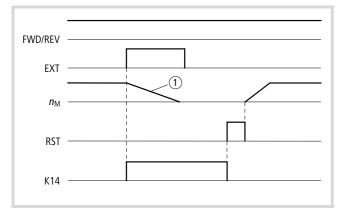
Figure 64: Function chart for EXT (external fault message)
