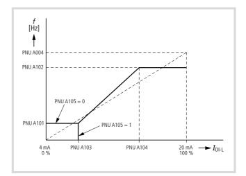
Figure 50: Setpoint current, terminals OI-L
