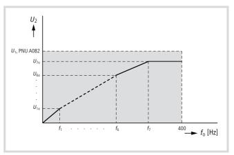
Figure 109: Limits of the freely adjustable UIf characteristic
