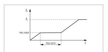
Figure 114: Function chart for acceleration waiting time
