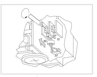
Figure 146: Disconnect J51 from terminals R0 and T0
