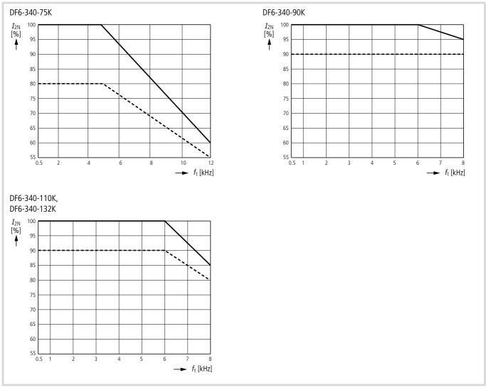
Figure 152: Derating curves, DF6-340-75K to ...-132K
