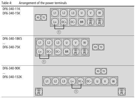
① Internal connection. Remove if a DC link choke is used.
