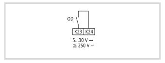
Figure 95: Relay output K23-K24 configured as OD (PID control deviation)
