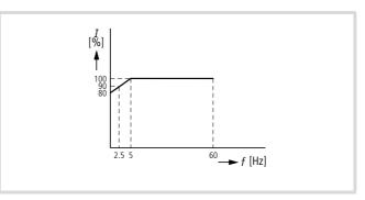
Figure 137: Normal overload protection (PNU b013 = 01)
