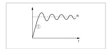
Figure 119: Oscillation, dampened
