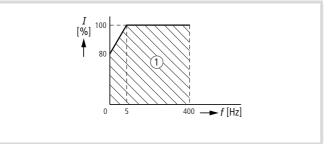
Figure 141: Setting range for the adjustable overload protection
