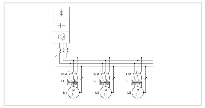
Figure 31: Parallel connection of multiple motors
