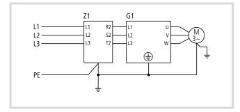
Figure 12: Earthing measures Z1: RFI filter G1:Frequency inverter
