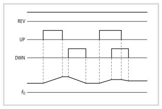
Figure 74: Function chart for UP/DWN (acceleration/deceleration – motor potentiometer)
