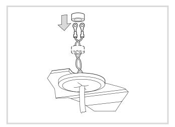
Figure 24: Push on the ferrite rings
