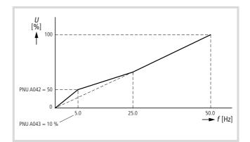
Figure 105: Voltage boost characteristics
