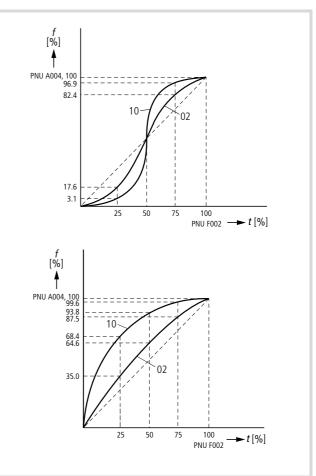
Figure 130: Curvature of the S- and U-curve characteristics
