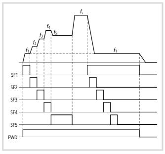
Figure 57: Function chart for bitwise fixed frequency selection (SF1 to SF5)
