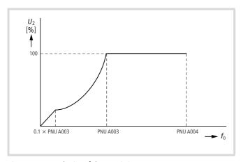
Figure 107: Quadratic *UIf* characteristic *U*<sub>2</sub>:Output voltage *f*<sub>0</sub>: Output frequency
