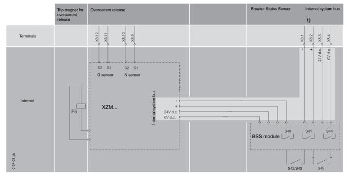
1)Terminating resistor on X8-1 / X8-2, when no external systembus module. ( $\rightarrow$  page 9 – 60)
