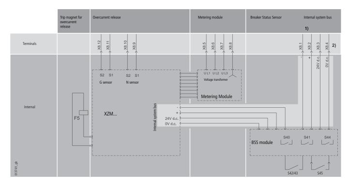
1) Terminating resistor on X8-1 / X8-2, when no external systembus module.
