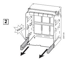
Place the circuit-breaker in the withdrawable unit and push it into disconnected position
