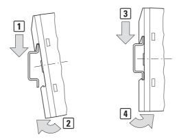
Figure 8: Mounting on top-hat rail
