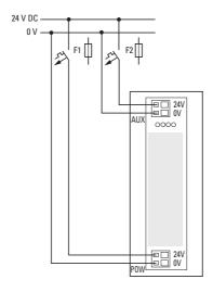
Figure 11: Connection of power supply
