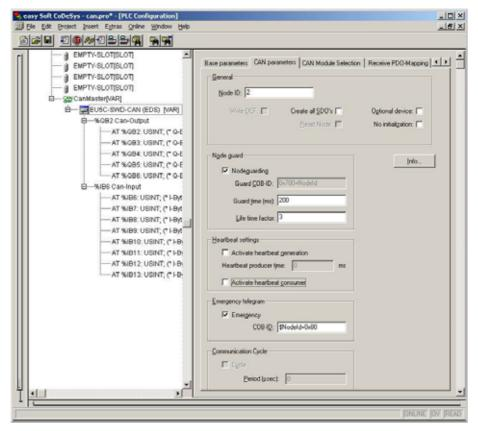
Figure 21: Adjusting the CAN parameters in XSoft-CoDeSys-2
