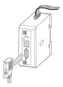
Figure 13: EtherNet/IP or Modbus-TCP CANopen
