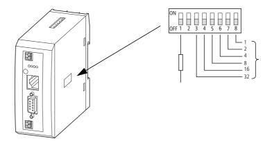
Figure 5: Activate the EU5C-SWD-CAN bus termination resistor
