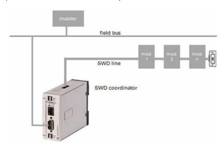
Figure 1: Connecting the field bus and SmartWire-DT with a gateway
