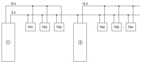
Figure 25: Schematic layout of an SWD line with the EU5C-SWD-PF2 power feeder module
