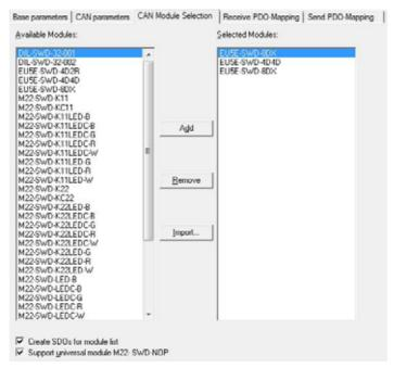
Figure 18: Selection of SWD modules in XSoft-CoDeSys-2
