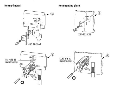
Figure 15: Field bus shielded by using a shield
