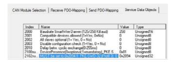
Figure 20: Entering profile code "0x2094" into the "Value" column
