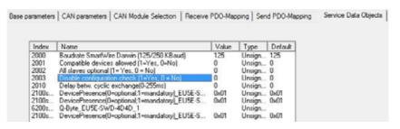
Figure 19: Setting "Disable Configuration check" to "1" in XSoft-CoDeSys-2
