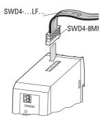
Figure 12: Connection SmartWire-DT
