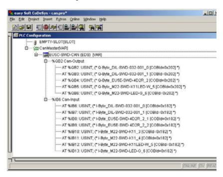
Figure 23: SWD module addresses in XSoft-CoDeSys-2
