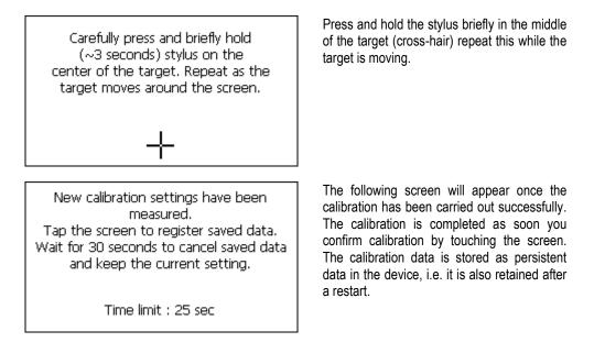
With the additional parameter "Touch.exe -r -q" you can prevent that an additional message about the success of the calibration is displayed. In this mode, the program has a return value to indicate the state of the calibration (true: success, false: failed).
