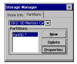
When a new partition is created, the maximum available memory space can be used, or the size can be defined in the number of sectors. MBs are converted into sectors as follows:
