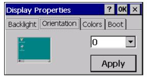
Display orientation can be set with the «0» (default setting) or «90» settings. The display is rotated in a clockwise direction. The «90» setting should be selected for vertical mounting. The picture on the left of the dialog shows the orientation set. The setting is not transferred until after a restart.
