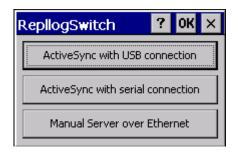
The «Repllogswitch.exe» program is used for establishing a connection with a PC via «ActiveSync» or «Manual Server». This is described in the chapter <u>Procedure: ActiveSync</u> or <u>Procedure: Manual Server</u>.
