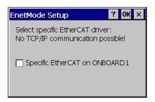
You can configure the ethernet interface as a EtherCAT interface here. If it is in EtherCAT mode, no TCP/IP communication via this interface can take place!
