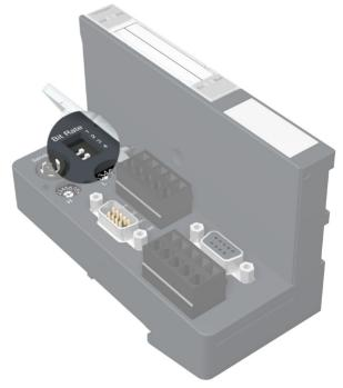
Figure 16: DIP switches to set the transfer rate
