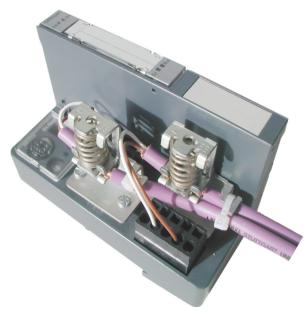
Figure 7: Shielding connection for an XN-GW-CANopen
