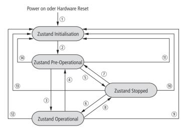
Figure 30: Boot procedure with Minimum Boot-up
