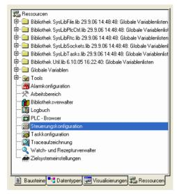
Figure 33: Selecting PLC configuration
