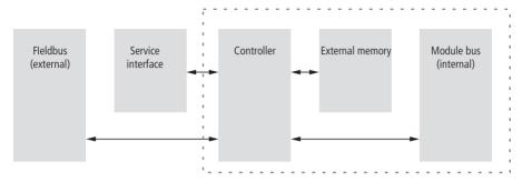
Figure 20: Structure of a XNE-GWBR-CANopen
