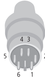
Figure 11: PS/2 plug on connecting cable to the gateway (plan view)
