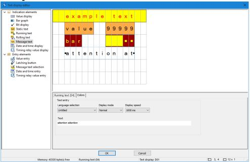
If you want to display a text that is longer than 16 characters, you can use the running text display element. This option can come in particularly handy when you want to draw the machine operator's attention to a text.
