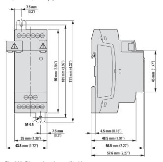
Fig. 368: Dimensions in mm (Inch)
