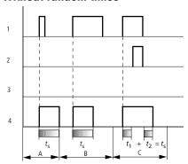
Fig. 149: Signal diagram timing relay, single pulse 1
