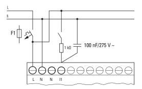
Fig. 7: Limitation of the input current through resistors
