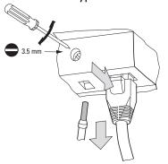
Fig. 38: Removing the Ethernet cable
