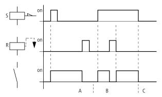
Fig. 98: Set and Reset signal diagram
