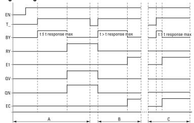
Fig. 251: Signal diagram of frequency counter
