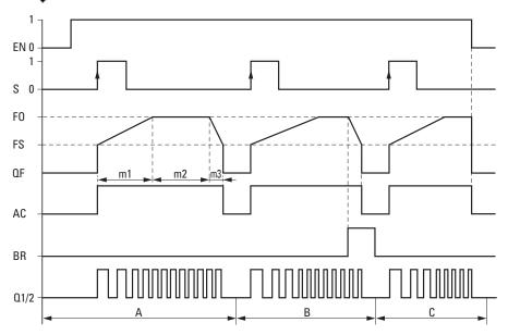
Fig. 198: Signal diagram for PO pulse output with specified number of pulses for I1 - possible normal mode phases
