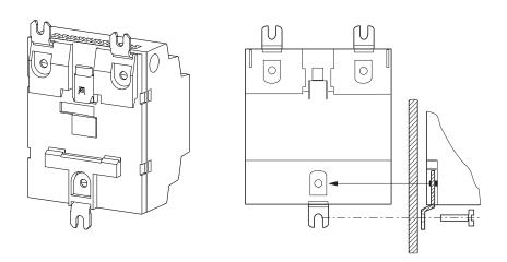
Fig. 14: Example: Screw mounting for a 4U device
