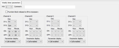
Fig. 126: Programming view Weekly timer parameters tab
