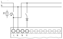
Fig. 4: AC input with suppression diode easyE4 AC
