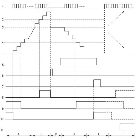
Fig. 171: Signal diagram of counter relay
