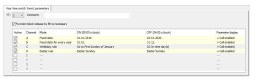
Fig. 154: Year time switch (new) parameters tab for YT function block with example showing all four modes
