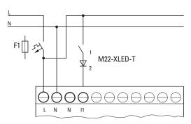
Fig. 5: AC input with ballast M22-XLED-T
