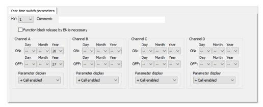
Fig. 136: Year time switch parameters tab with and example in which a year range is being selected
