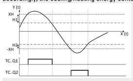
Fig. 204: Signal diagram for three-step controller
