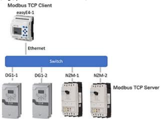
Four Modbus TCP server modules are allowed per base device.
