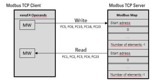
Fig. 238: Overview of how function codes are used
