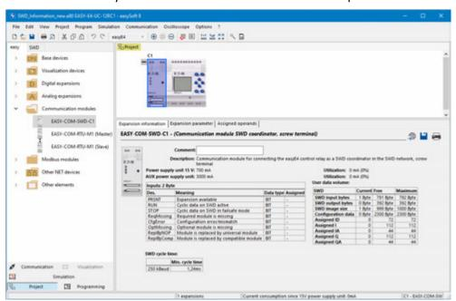
Fig. 344: Work pane with base device and communication module; catalog expanded with "SWD" tab
