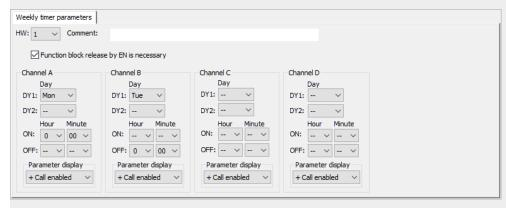
Fig. 134: Programming view Weekly timer parameters tab - 24 hours setting
