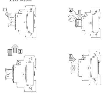
Fig. 35: Removing the memory card
