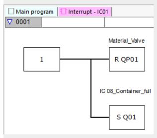
Fig. 260: easySoft 8 Interrupt program, two counter inputs
