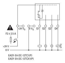
Fig. 24: Connecting base device transistor outputs
