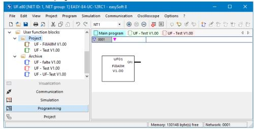
Fig. 283: easySoft 8 with function blocks in list of operands and function blocks, User function block/Project directory and User function block/Archive directory with UF-BETest V1.00 versions with different contents
