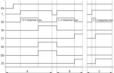
Fig. 241: Signal diagram of frequency counter
