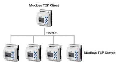
Fig. 351: One easyE4 functioning as a Modbus TCP client controlling four Modbus TCP servers
