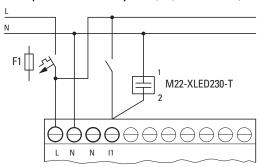
Fig. 8: An increase in input current with M22-XLED230-T
