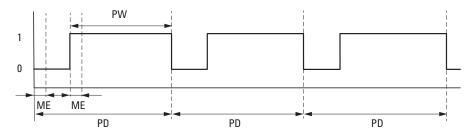
Fig. 189: PW pulse at the function block output when SV = 3218, ME = 93 ms, PD=1000 ms
