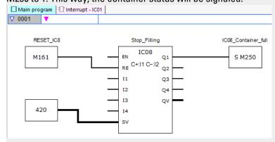
Fig. 259: easySoft 8 Main program, two counter inputs
