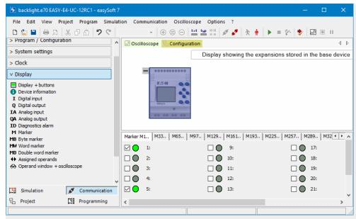
Fig. 304: Online Communication view with display marker, causing the device display to flash green
