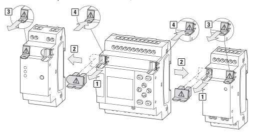
Fig. 15: Remove adjacent connectors
