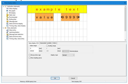
Value displays can be very effectively combined with a static text. In the example above, the value display element has been placed to the right of the "Value" text in the preview pane. The display in the example is intended to have five digits, which is why the number of characters has been configured accordingly. (The number 9 symbolizes value displays.)
