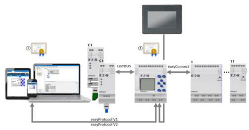
Fig. 311: easyE4 communication diagram
