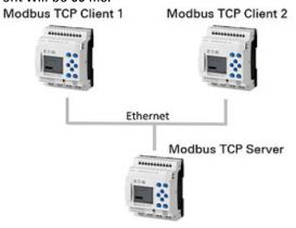
Fig. 350: A single easyE4 functioning as a Modbus TCP server handling two Modbus TCP clients
