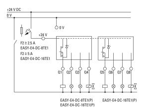
Fig. 25: Connecting expansion device transistor outputs
