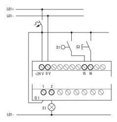
Fig. 290: Wiring with EASY-E4-UC-..., for example
