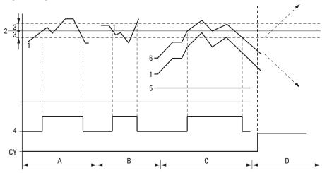
Fig. 177: Analog comparator signal diagram
