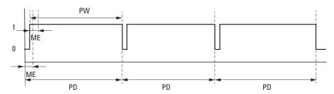
Fig. 190: A constant signal is signaled at the function block output when SV = 3768, ME = 93 ms, PD=1000 ms; E1 = 1
