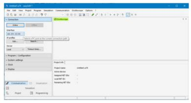
Fig. 68: Selecting the easyE4 device's IP address
