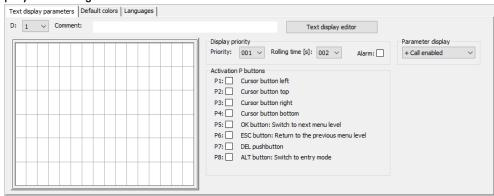
Fig. 222: Text display parameters tab for text display function block in the Programming view
