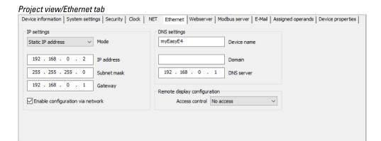
Fig. 336: Ethernet tab with settings from the example
