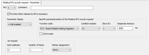
Fig. 247: Acyclical Modbus RTU request - Parameters tab
