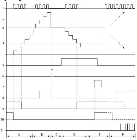
Fig. 176: Signal diagram High-speed incremental value counter
