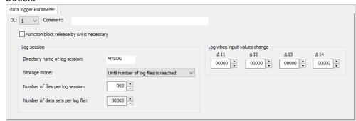
Fig. 235: Data logger tab with set parameters for the programming view
