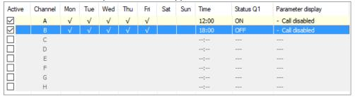
Fig. 161: Weekly timer (new) parameters tab with an example
