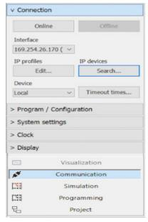
Fig. 65: Establishing an Ethernet connection
