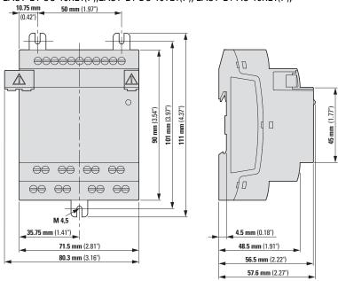
Fig. 366: Dimensions in mm (Inch) extensions 4SU
