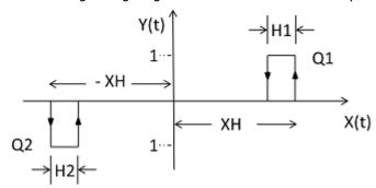
Fig. 203: Timing diagram for three-step controller
