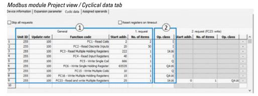
Fig. 356: Cyclical data tab with sample function codes that have been configured and added range boxes
