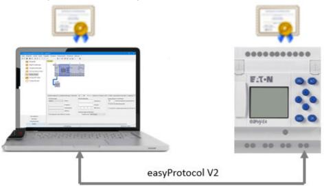
easyProtocol V2, SSL/TLS comes enabled by default on easyE4 base devices with firmware version ≥ 2.00. This ensures that communications can only be established in an encrypted manner with easyProtocol V2 with new devices, which additionally requires the Eaton easyE4 root certificate. If this certificate has been installed on the same PC on which easySoft 8 is running, secure communications will be established through the programming interface.
