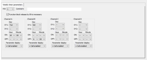
Fig. 130: Programming view Weekly timer parameters tab
