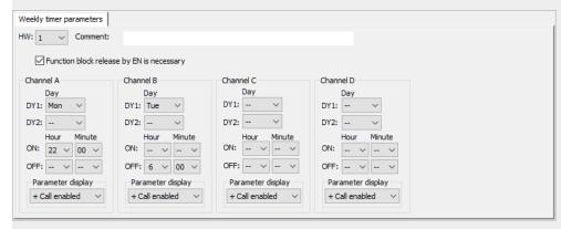
Fig. 135: Programming view Weekly timer parameters tab
