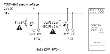
Fig. 342: EASY-COM-SWD-...Connecting the power supply
