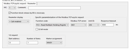
Fig. 237: Acyclical Modbus TCP request - Parameters tab
