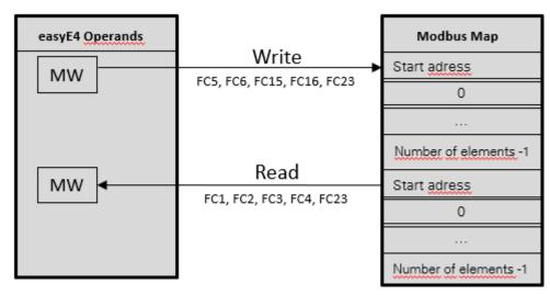
Fig. 248: Overview of how function codes are used
