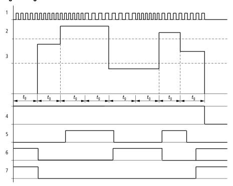
Fig. 172: Signal diagram of frequency counter
