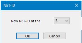
Fig. 318: NET-ID dialog box used to assign a NET ID when adding a new base device
