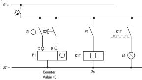
Fig. 289: Hardwiring with relays
