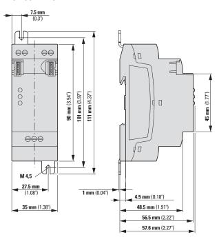
Fig. 370: Dimensions in mm (Inch) extensions 2SU
