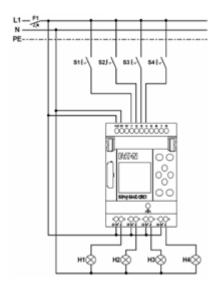
Fig. 371: Circuit diagram for easyE4 chaser light
