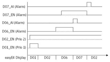
Fig. 225: Signal diagram Text display
