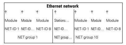
NET uses UDP protocols that send unconfirmed broadcast frames; accordingly, the devices in the NET group must be located on the same subnet. Connections through a router are not allowed, as broadcast frames will normally be unable to pass through a router.
