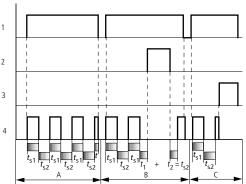
Fig. 151: Signal diagram timing relay, single pulse
