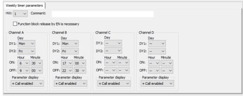
Fig. 128: Programming view Weekly timer parameters tab
