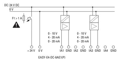
Fig. 28: Connecting analog inputs EASY-E4-DC-6AE1(P)
