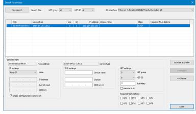
Fig. 67: Saving the found device's IP profile
