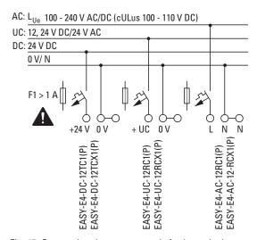
Fig. 17: Connecting the power supply for base devices
