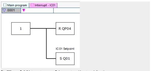
Fig. 258: easySoft 8 Interrupt program Pulse counter with external direction
