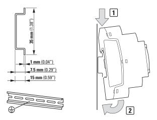
Fig. 12: Installation on IEC/EN 60715 mounting rail
