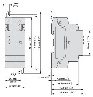
Fig. 369: Dimensions in mm (Inch) extensions 2SU
