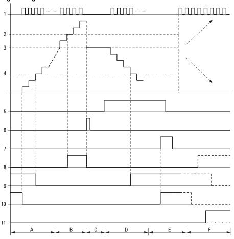
Fig. 173: Signal diagram High-speed counter
