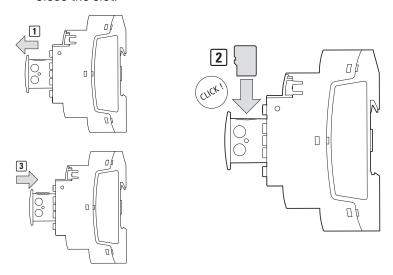
Fig. 34: Inserting a memory card
