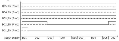
Fig. 226: Signal diagram for text display with text function blocks with an identical priority of 3
