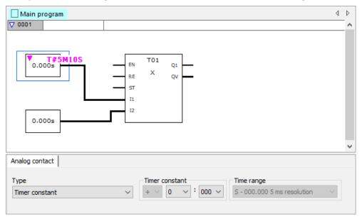
Fig. 122: Programming view: Selected timer constant on function block input I1 and unconfirmed value of <t#5m10s> entered with the keyboard
