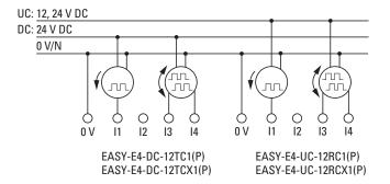
Fig. 21: Connect digital counter inputs
