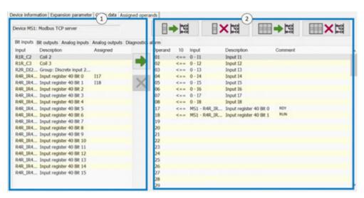
Fig. 358: Assigned operands tab after defining FC1, FC2, and FC4; bit inputs R4R\_IR40x0 and R4R\_IR40x1 have already been assigned to base device operands I17 and I18.
