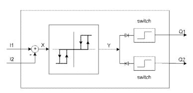
Fig. 202: Three-step controller schematic diagram
