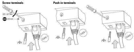
Fig. 37: Connecting the Ethernet cable
