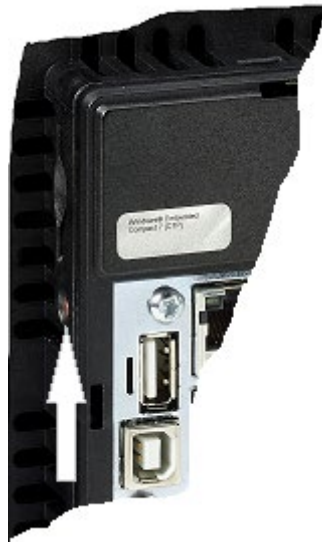
Figure 21: CTRL button on the side of the touch panel
