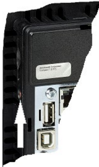
Figure 4: CTRL button on the side of the touch panel
