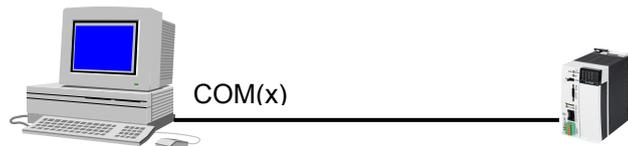
For the connection between the PC and PLC use a communication cable as described in the section "SYSTEM PORT and PC COM(x) variants".
