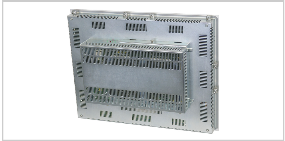
Abb. 44 15" devices with twelve retaining brackets (meet IP65 requirements)
