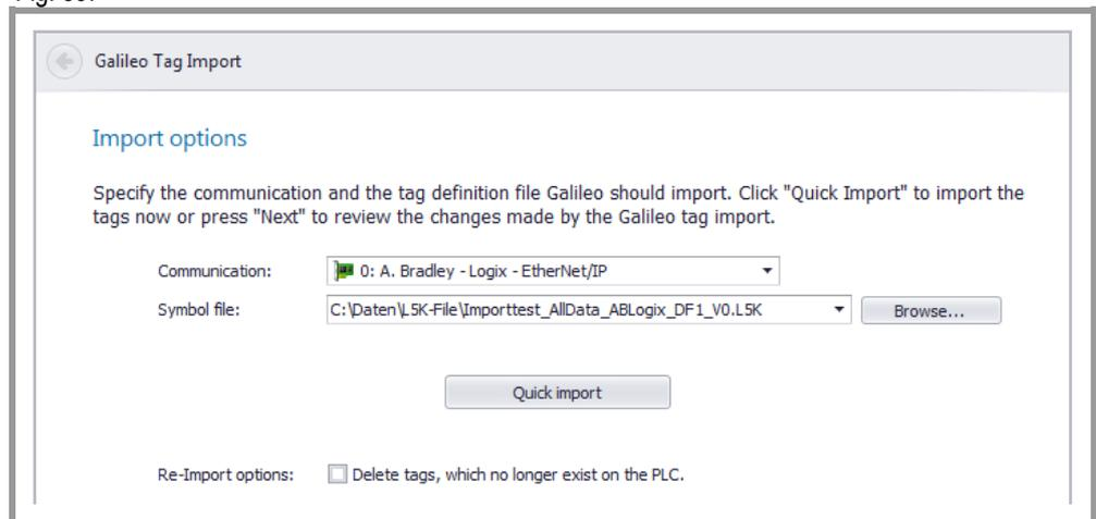
Fig. 39 Example of how to import a L5K tag information file into Galileo
