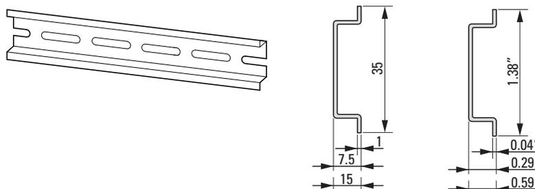
Figure 28: Mounting rail conforming with IEC/EN 60715
