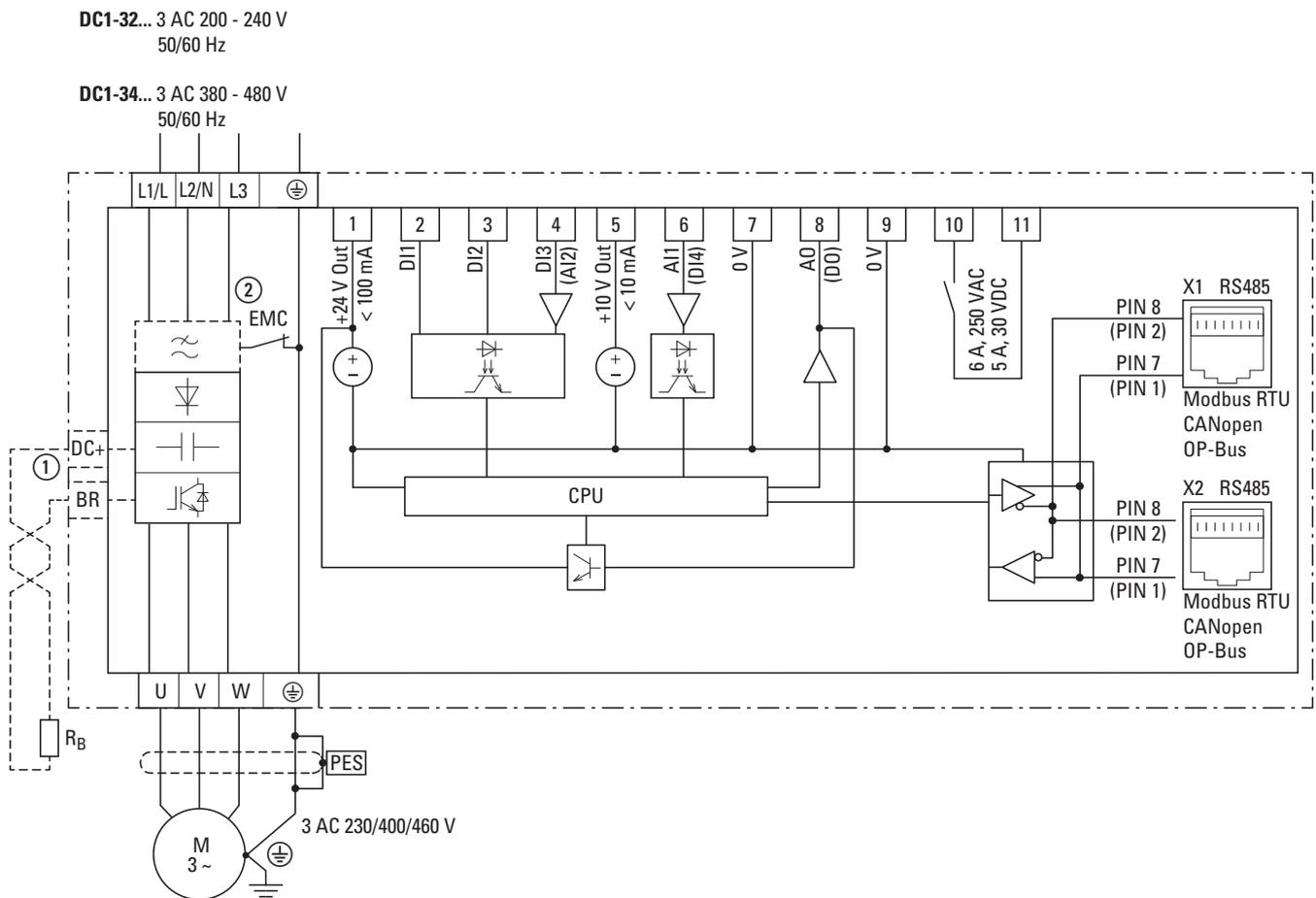
Figure 72: Block diagram DC1-32...-A66..., DC1-34...-A66...
