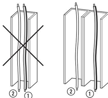
Figure 35: Separate routing
