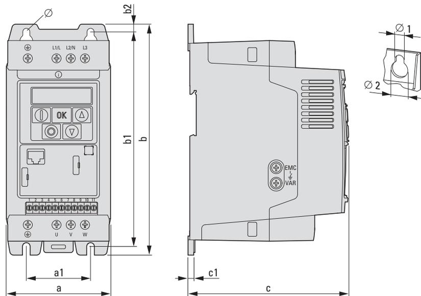
Figure 79: Dimensions for DC1 with IP20 degree of protection (NEMA 0)
