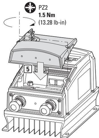
Figure 43: Removing the lower housing cover
