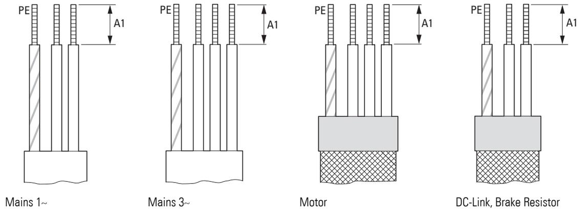
Figure 44: Stripping lengths in the power section
