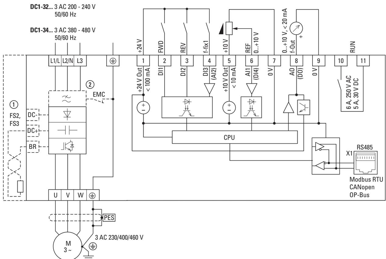
Figure 65: Block diagram DC1-32... and DC1-34... in frame sizes FS1, FS2 and FS3
