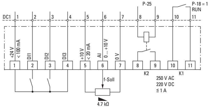
Figure 93: Block diagram DXC-EXT-2RO
