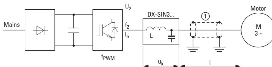
figure 88: Maximum permissible motor cable lengths
