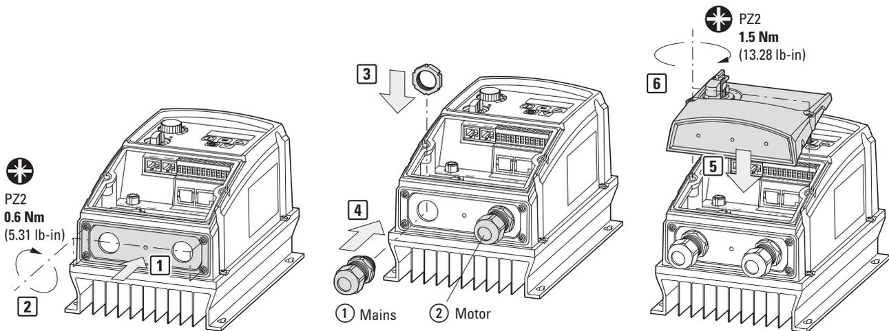
Figure 50: Installing the cable glands
