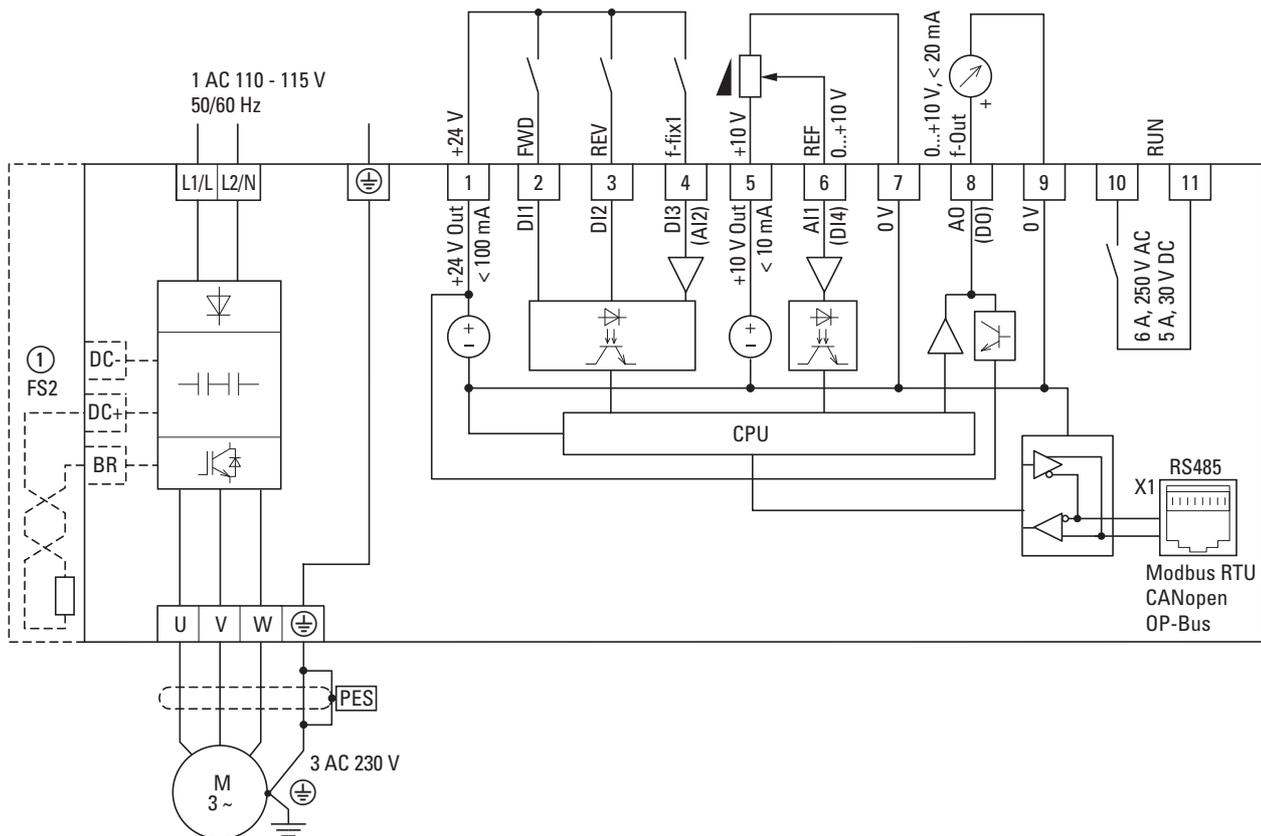
Figure 63: Block diagram DC1-1D...Nx...
