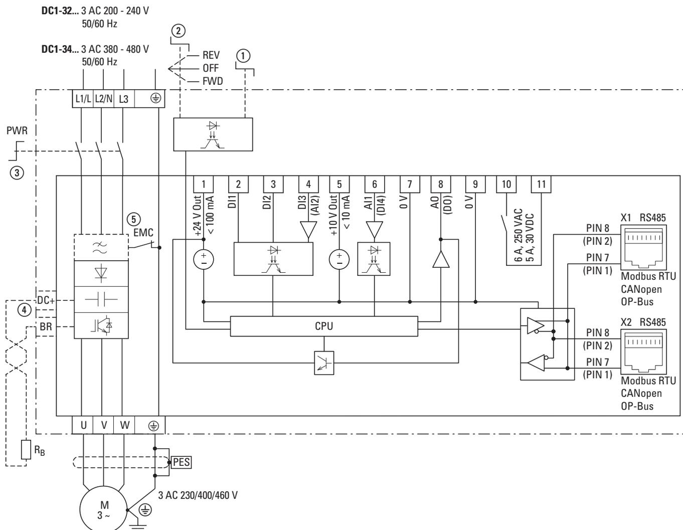
Figure 71: Block diagram DC1-32...-A6S..., DC1-34...-A6S...
