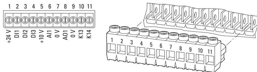
Figure 52: Control signal terminal layout and factory designations
