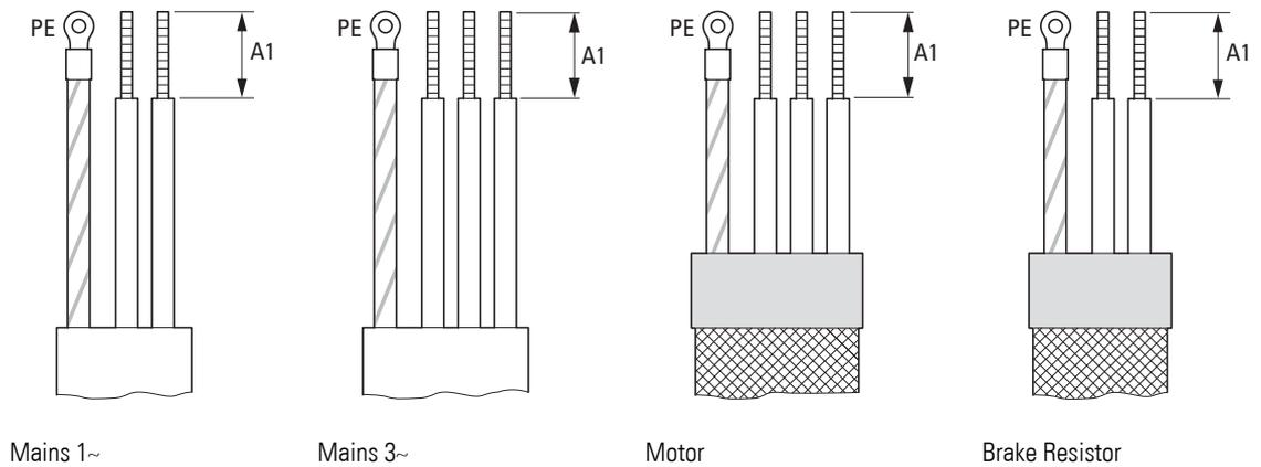
Figure 45: Stripping lengths in the power section
