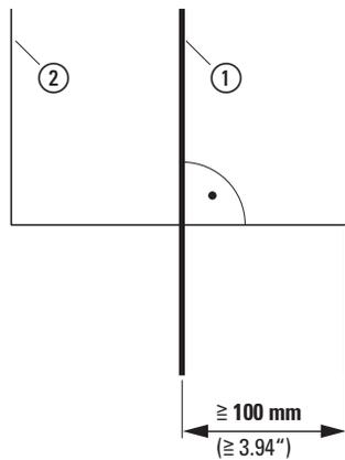
Figure 34: Cable routing
