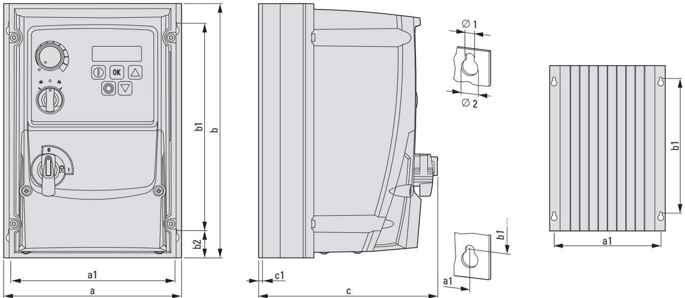
Figure 81: Dimensions for DC1 with IP66 degree of protection (NEMA 4X)
