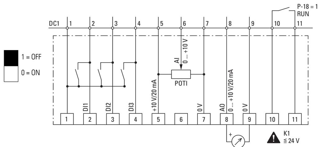
Figure 97: Block diagram DXC-EXT-LOCSIM simulator
