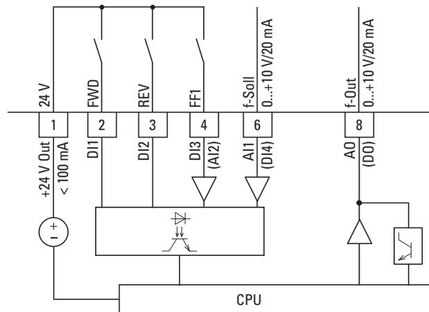
Figure 55: Control signal terminals (D = digital/A = analog)
