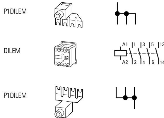
Figure 82: Mains contactor at single-phase connection (DC1-12...)
