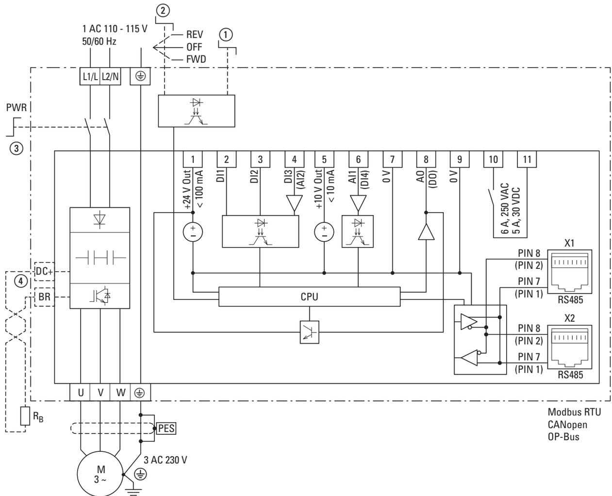
Figure 67: Block diagram DC1-1D...Nx-A6S...
