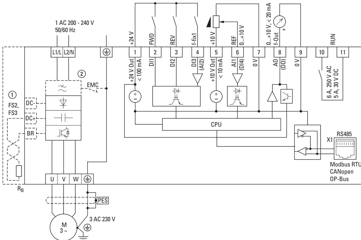
Figure 64: Block diagram DC1-12...
