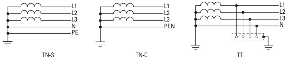
Figure 14: AC supply systems with earthed center point
