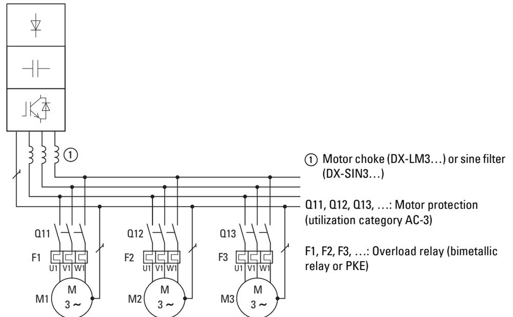
Figure 19: Example: Parallel connection of several motors to one variable frequency drive
