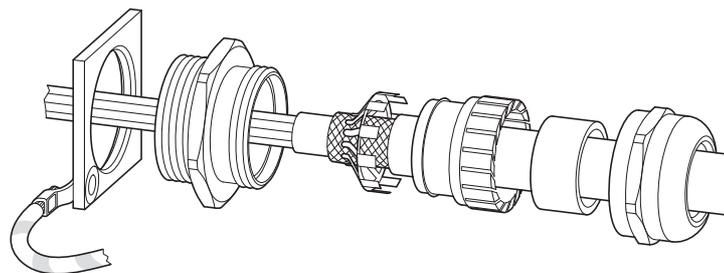
Figure 51: Example: diagram of EMC gland assembly
