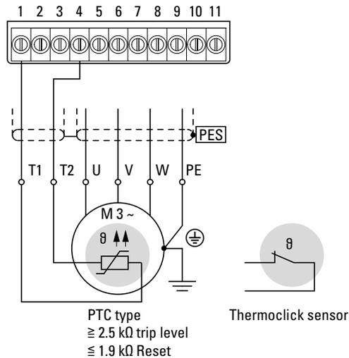
Figure 62: Thermistor connection
