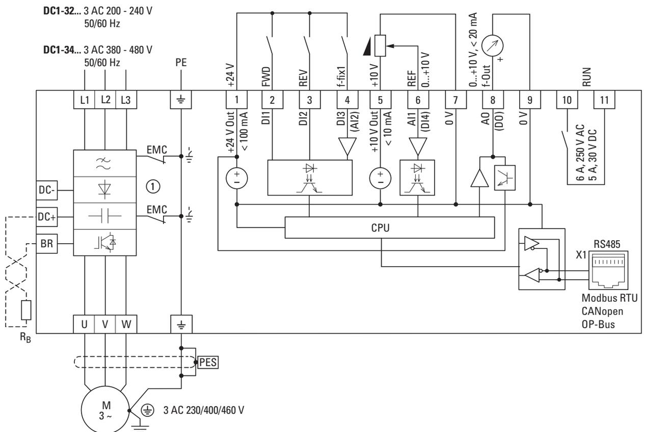
Figure 66: Block diagram DC1-32... and DC1-34... in frame size FS4
