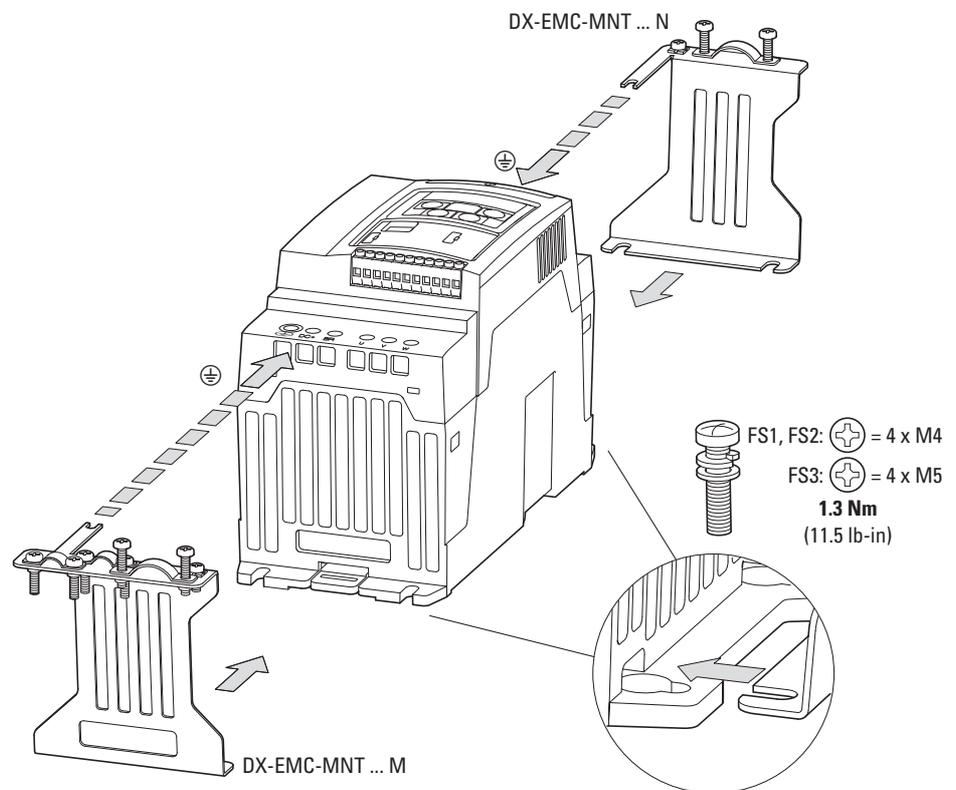
Figure 40: EMC cable brackets (example: FS2 frame size)
