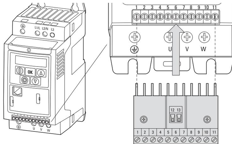
Figure 89: Connecting DXC... to the control signal terminals on the DC1 variable frequency drive
