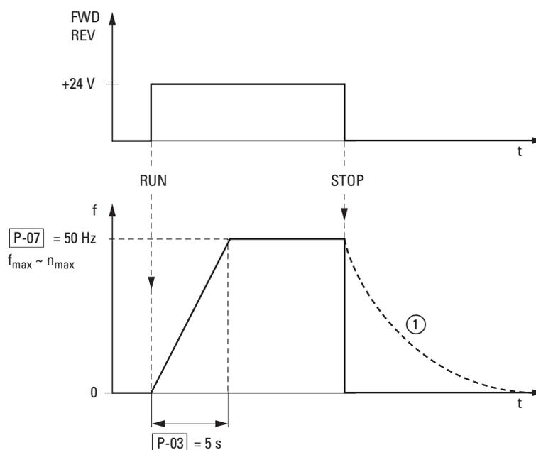
Figure 73: Start-Stop command with maximum reference voltage, acceleration ramp 5 s
