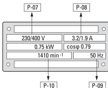
Figure 78: Motor rating plate, P-08 = 1.9 A at 400 V
