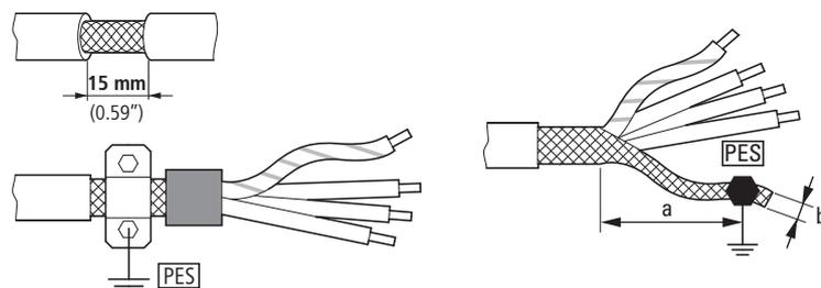
Figure 47: Screened connection cable in motor circuit
