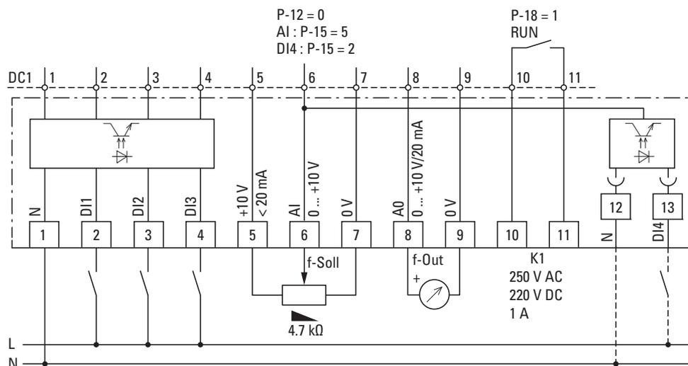
Figure 91: Block diagram DXC-EXT-IO110 and DXC-EXT-IO230
