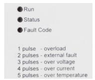
The LEDs on the front of the Variable Speed Starter indicate operating status and faults
