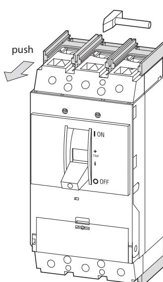
The barrier (shown shaded in the diagrams) is held tightly into grooves on top and bottom sides of the breaker or switch and must be removed in order to mount ...-XKA... Mechanical (Tunnel) lug connectors on NZM2 and NZM3 Circuit-Breakers and switches.
