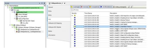
Device tree: Errors visible even at collapsed device tree
